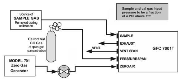
Figure 9-4: Pneumatic Connections – Option 50B: Ambient Zero/Pressurized Span Calibration Valves
